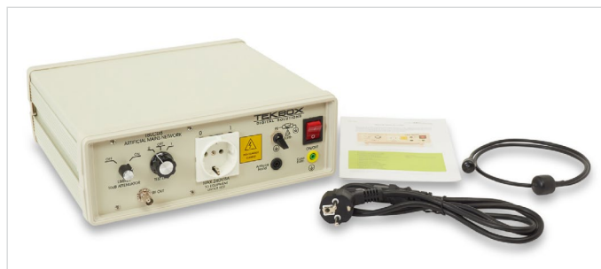
Figure 5. A typical line impedance stabilization network (LISN) used to couple conducted EMI from line cords to the spectrum analyzer. Photo, courtesy Tekbox Digital Solutions.
