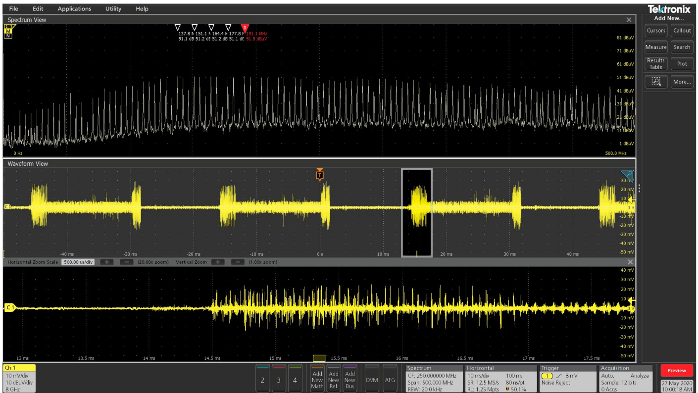
Figure 9. When Spectrum Time is moved over to the noisy digital burst in the time domain, the EMI increases by 20 dB. With Spectrum Time, it's possible to analyze whether this pulse of EMI can couple to cables and radiate.
