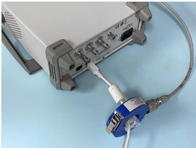
Figure 3. Use a current probe to measure high frequency currents flowing on I/O and power cables.
