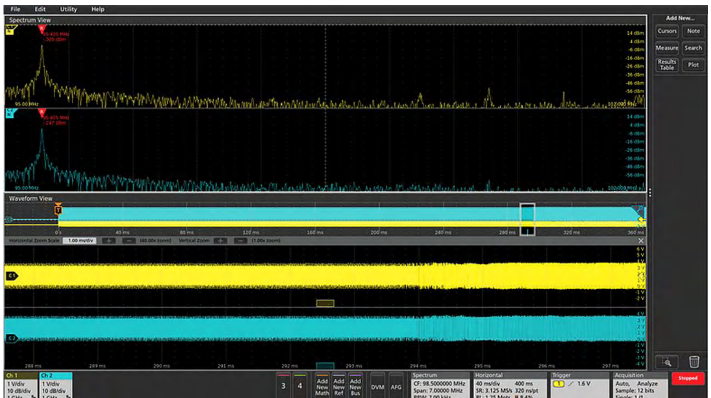
Figure 17. When debugging tasks demand it, multiple channels can be analyzed simultaneously. Here, two channels show the startup of a clock signal from two different points in a circuit.
