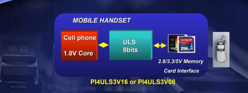
Application: Data/Address bus voltage translation between 1.8V Baseband SOC and Memory Card.
