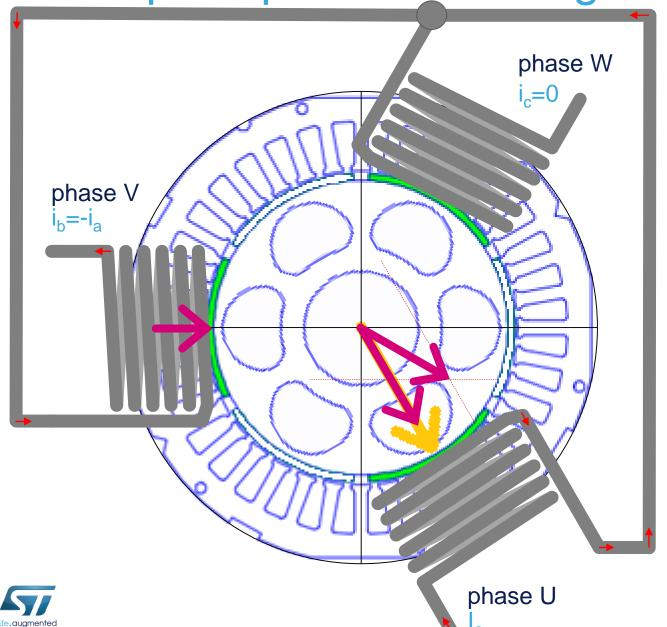
Stator coils are connected in the neutral point, only 3 terminals U, V, W are needed
