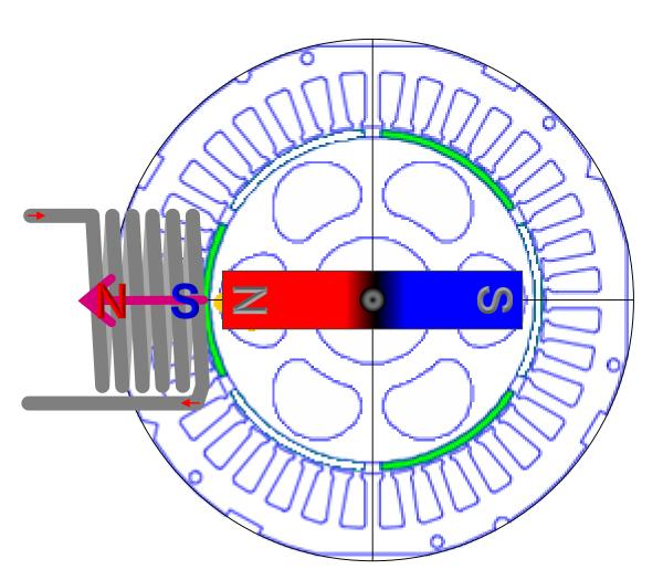
Magnetic fields of the rotor and coil can be described by vectors (with their size and direction, or x-y coordinates)
