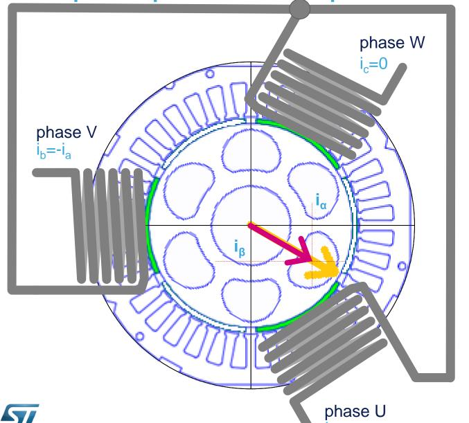
Lock of axial system to rotor position
