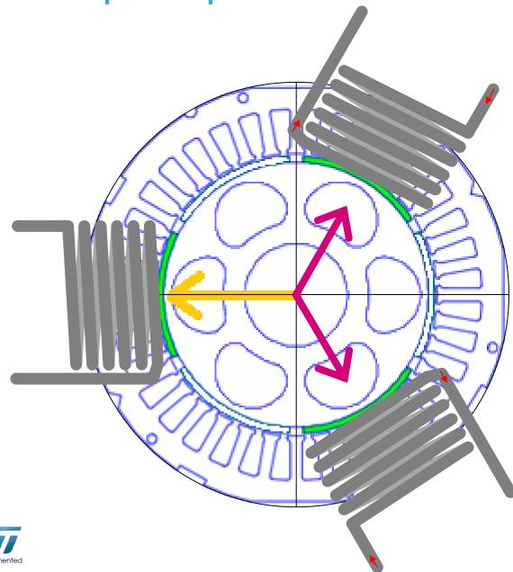
Second coil Current applied to this coil causes rotor to move again Third coil Current applied to this coil causes rotor to move yet again
