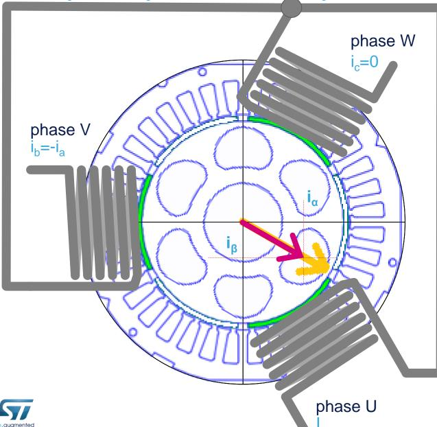
Lock of axial system to rotor position
