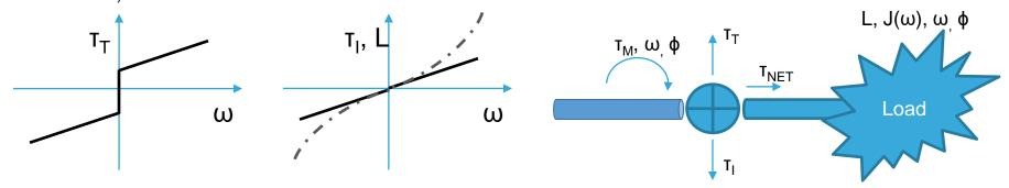
•  $T_{NET} = J(\omega) \frac{d\omega}{dt}$  is load torque, typically non-linear • Thus  $\omega(t) = \int_{\tau_0}^t \frac{\tau_{NET}(t)}{J(t)} dt + \omega_0$
