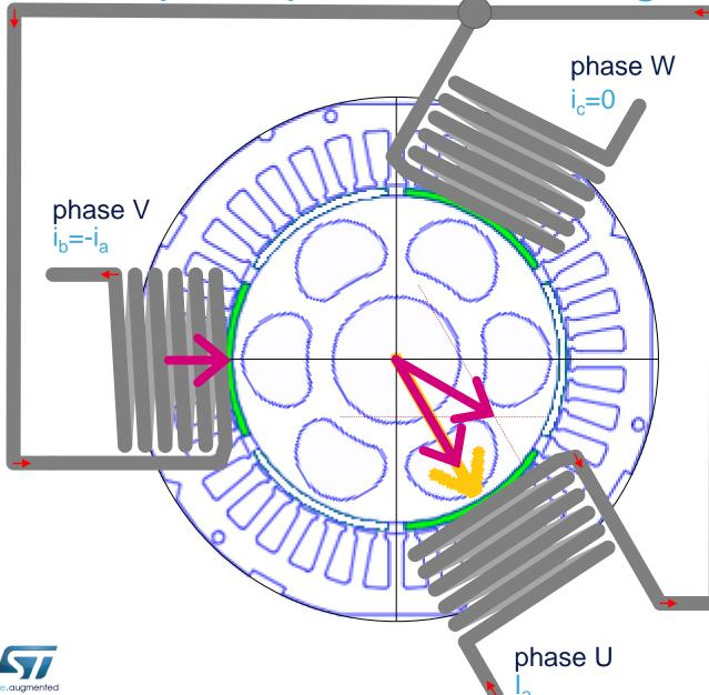
Stator coils are connected in the neutral point, only 3 terminals U, V, W are needed
