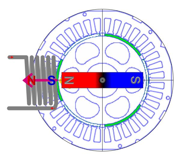
Magnetic fields of the rotor and coil can be described by vectors (with their size and direction, or x-y coordinates)
