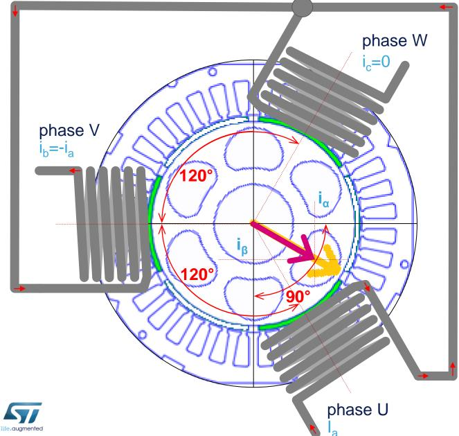
transforms  $i_a, i_b, i_c (120^\circ)$ to  $i_{\alpha}, i_{\beta} (90^\circ)$
